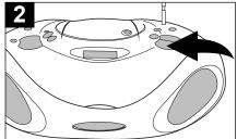
During CD playback, if you wish to pause the disc momentarily, press the PLAY/PAUSE (►■ )/ MEM-UP button. Playback stops but the disc continues to spin and the track number blinks in the display.
